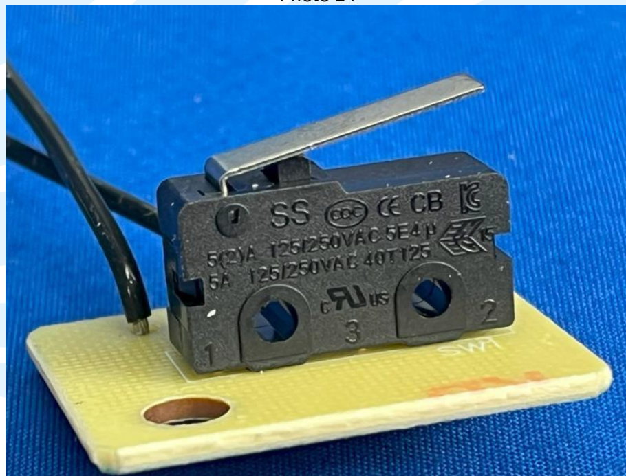
Description: Interlock switch - CY01, CY02, CY03
