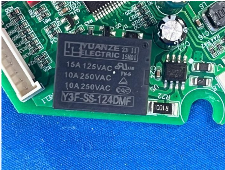
Description: Relay (REL1) - CY01, CY02, CY03
